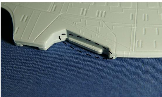
To ensure a good fit, the alignment tabs on the upper main saucer (kit part #1) will need to be removed. These are the protrusions in the part that are designed to align the original impulse engine parts (see illustration).
